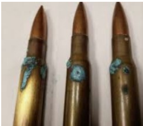
Corrosion of the brass cartridge case can often be caused by breakdown of the propellant.
